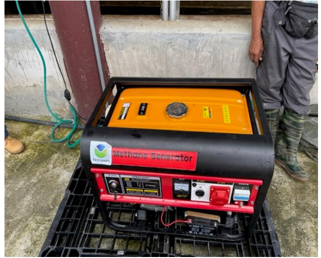
Methane fermenter and methane generator to generate electric from cattle waste
